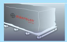
1 | The sheets should be stored flat and indoors, wherever possible. If stored outside, cover the Makrolon® multi UV sheets with white polyethylene (PE) sheeting. The chosen supporting structure must be nonwarping. Laminated timber beams or metal supporting structures with longitudinal rafters, on which the glazing bars are mounted, are the ideal choice.
