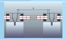
4 | The clear width or sheet width (B) of Makrolon® multi UV sheets is calculated from the rafter spacing, the dimensions of the chosen glazing bars and the required allowance for expansion (3 mm/m for polycarbonate).
