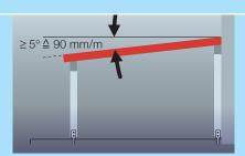
2 | We recommend a roof pitch of at least 5° (≙90 mm/m) to allow rainwater to flow off better. This has the benefits of maintaining seal integrity and the sheets are naturally cleaned by the rain.
