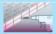
**7** | Swarf that has entered the sheet chambers can be blown out with compressed air or removed using a vacuum cleaner.
