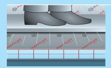
11 | Place the Makrolon® multi UV sheets on the purlins. It is important to place the side with UV protection facing outwards or upwards. This side is marked on the masking film and stamped along the sheet edge. Avoid walking on the sheets. If necessary, place a thick plank across the sheet.
