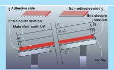
**5** | The correct order length (L) of Makrolon® multi UV sheets can be simply and safely determined, bearing in mind the following:
