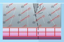
8 | If the sheet width of Makrolon® multi UV sheets has to be reduced, please cut as close as possible to the next web to ensure the best clamping action of the glazing bar.
