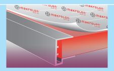
10 | When sealing sheet ends there is a simple, but very important, rule to follow which keeps condensation to a minimum: seal as tightly as possible at the top (e.g. seal edges with aluminium tape and if necessary affix an aluminium-end profile, possibly with seal), and as tight as necessary at the
