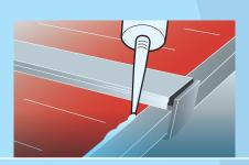
**14** | Seal the upper sealing strip of the end-closure section with silicone rubber that is compatible with Makrolon® and smoothen it out so that no water can enter.
