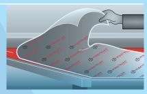
**13** | Finally, remove the masking film from the Makrolon® multi UV sheets. It should not be exposed to weathering for more than 24 hours.
